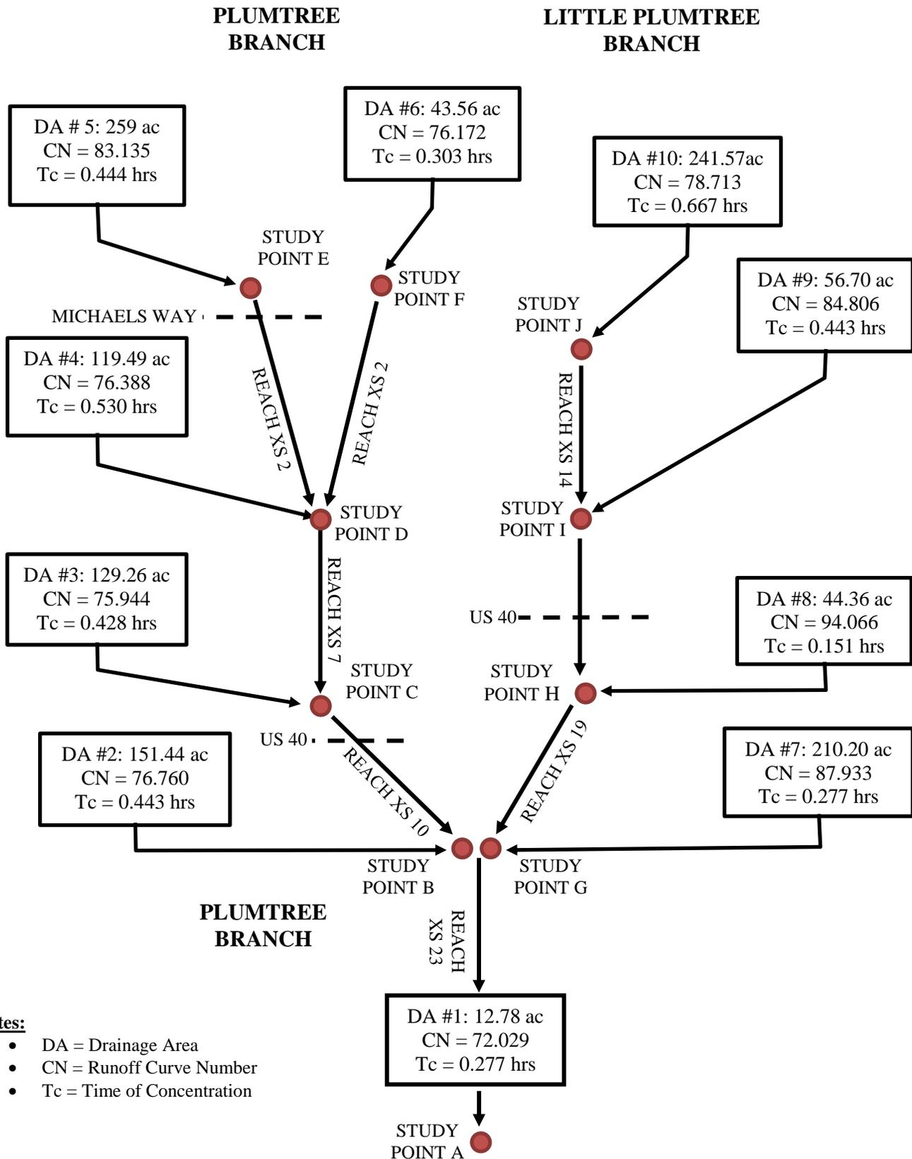
Figure 2.4: TR-20 Schematic for the Existing Conditions Hydrologic Analysis
