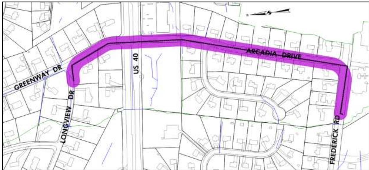
**Figure 4.4: Option D Storm Drain Extension from Greenway Drive**
