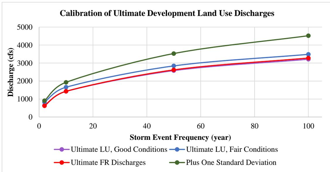
**Figure 2.3: Calibration Graph of Ultimate Land Use with Fixed Region Regression Equation Discharges**
