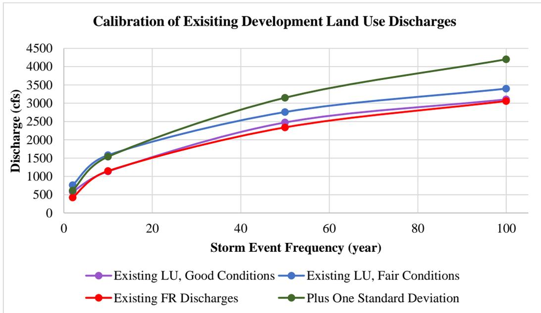
**Figure 2.2: Calibration Graph of Existing Land Use with Fixed Region Regression Equation Discharges**
