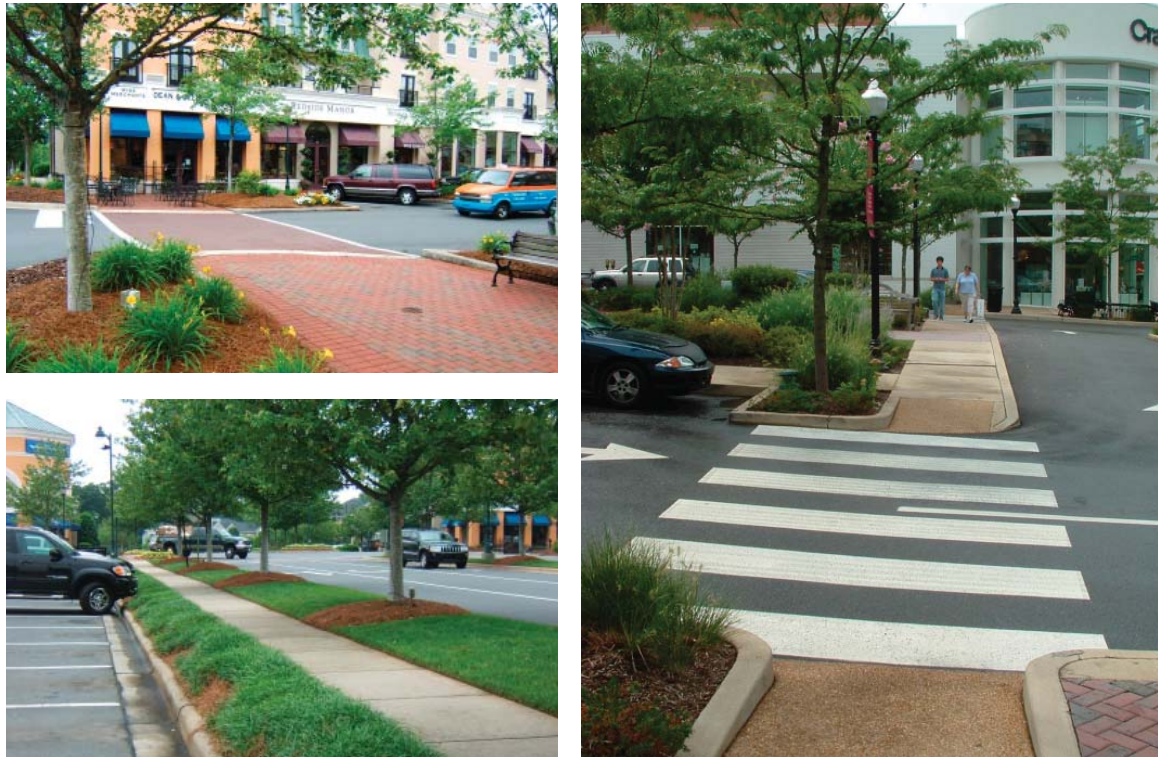
Figure 3L: The above photographs (top left and right) illustrate how crosswalks can reinforce pedestrian circulation patterns and provide visual clues to motorists that they are in a pedestrian-friendly environment. The photograph at the bottom left illustrates how well-located sidewalks can reinforce pedestrian routes even through parking areas.
