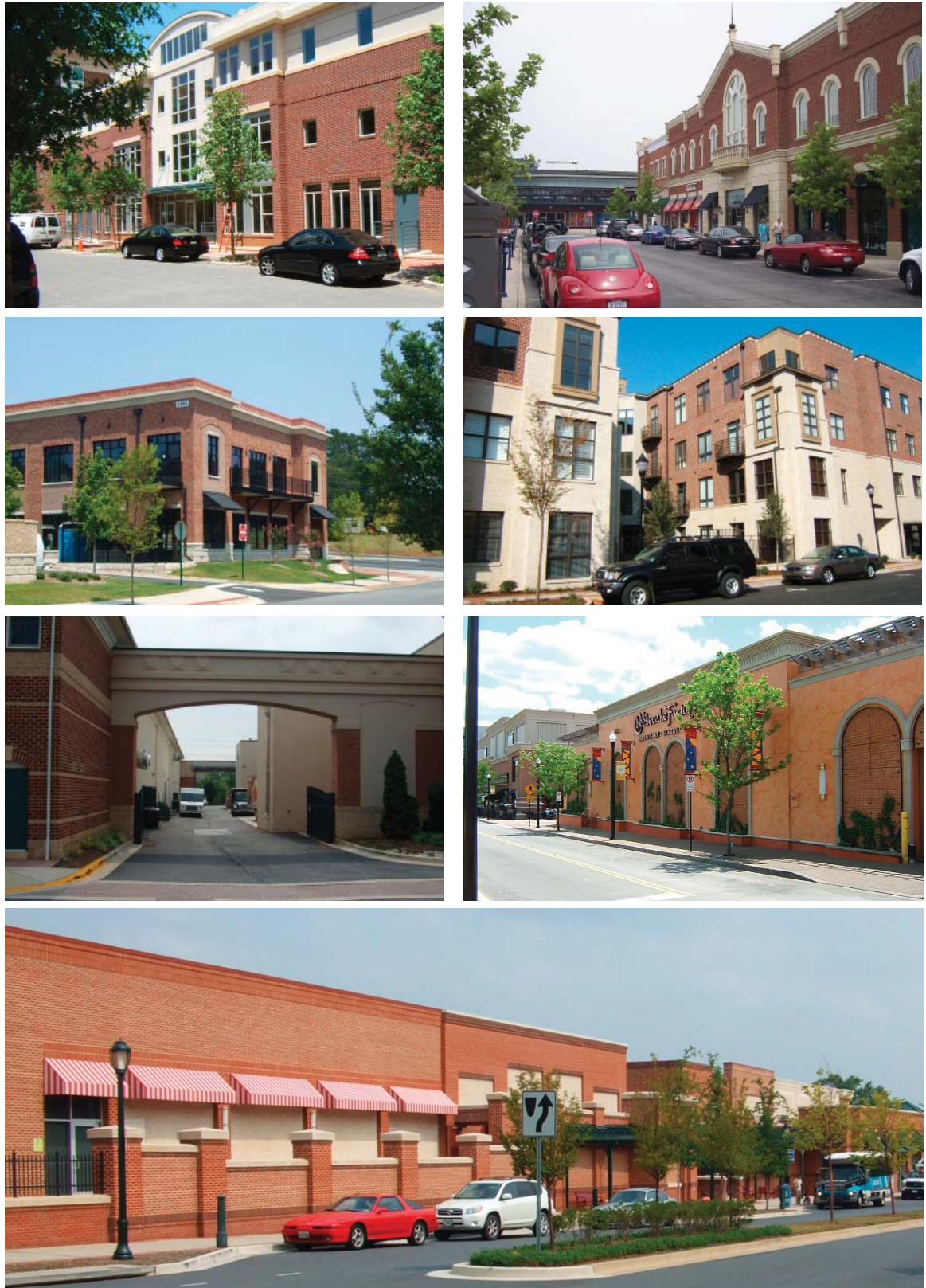
Figure 5D: Examples showing articulation of facades and roof lines, visual interest at the ground floor and articulation of blank walls facing streets.
