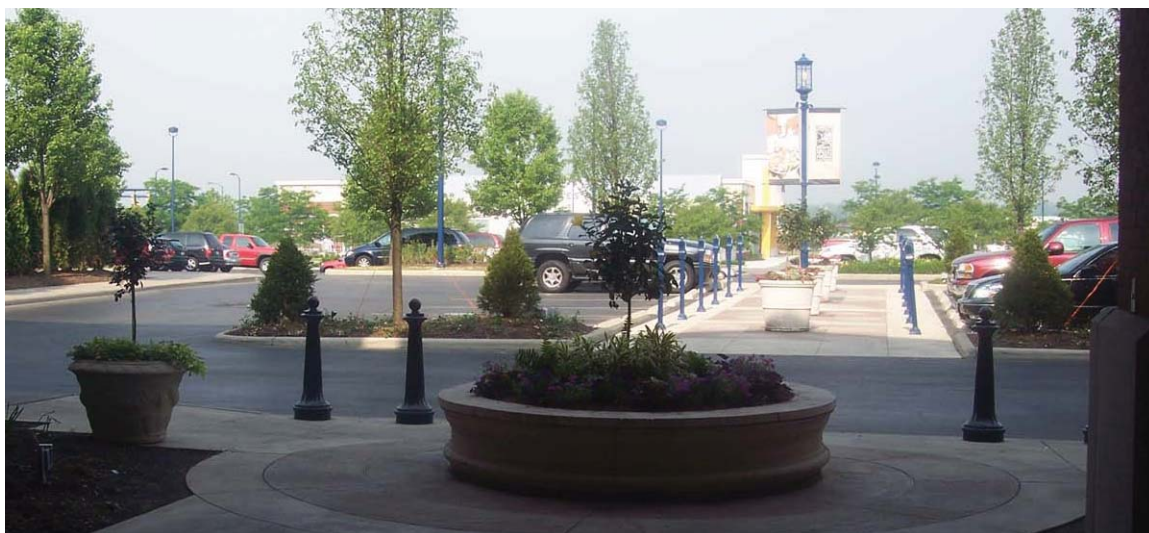
Figure 31: Examples of how parking islands can divide large parking areas into smaller “rooms” and how pedestrian access can be provided through and adjacent to parking areas.
