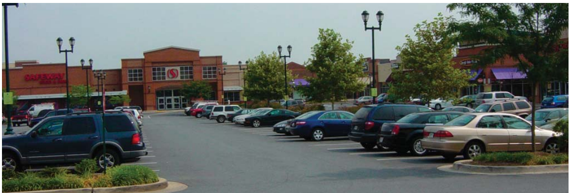
The photograph above illustrates how planted medians and canopy shade trees can be used to reduce the negative impacts of large areas of parking.
