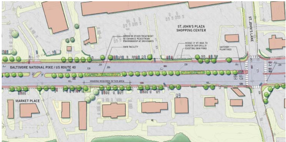
Plan View of Chatham Area showing typical improvements shown in the Streetscape Master Plan: sidewalks, crosswalks, street trees, median plantings and shrubs to screen parking.
