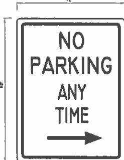
'R7-I NO PARKING' SIGN DETAIL NOT TO SCALE
