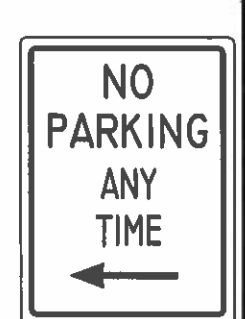
'R7-I NO PARKING' SIGN DETAIL NOT TO SCALE
