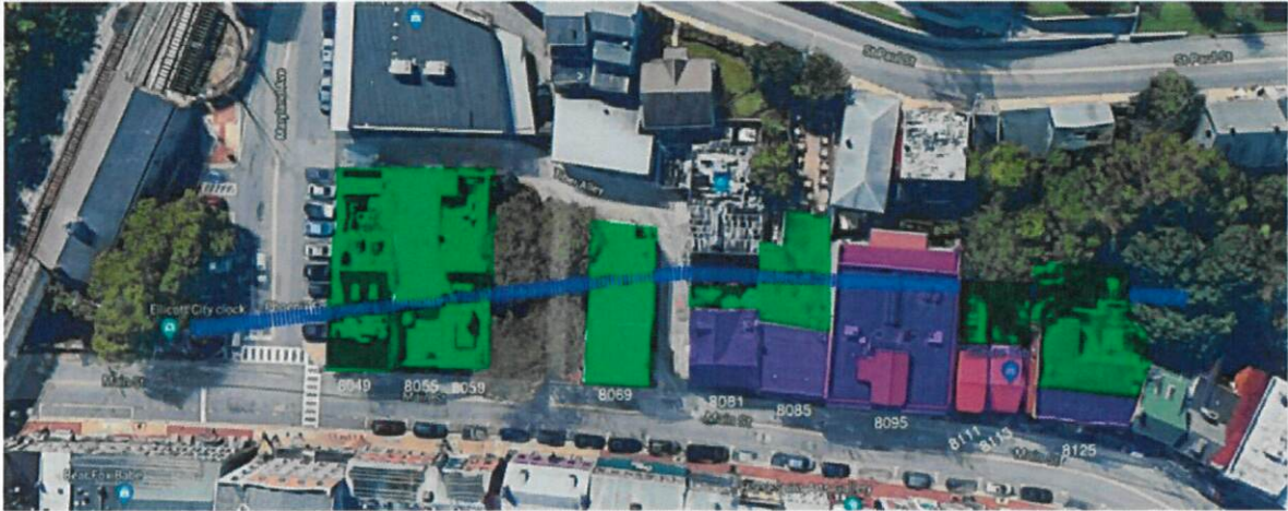
Figure 138: Howard County Acquired Ten Buildings on the South Side of Main Street. Under the EC Safe and Sound Plan, the Buildings or Rear Additions Shaded in Green Will Be Demolished (with Historical Building Components Salvaged) While Buildings Shaded Purple/Pink Will Remain. The Blue Line Indicates the Approximate Location of the Tiber Branch.
