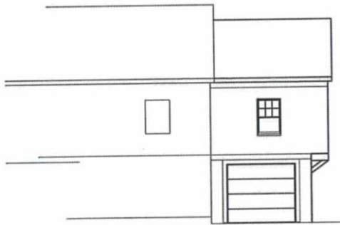
Figure 12 - Proposed front elevation of addition
