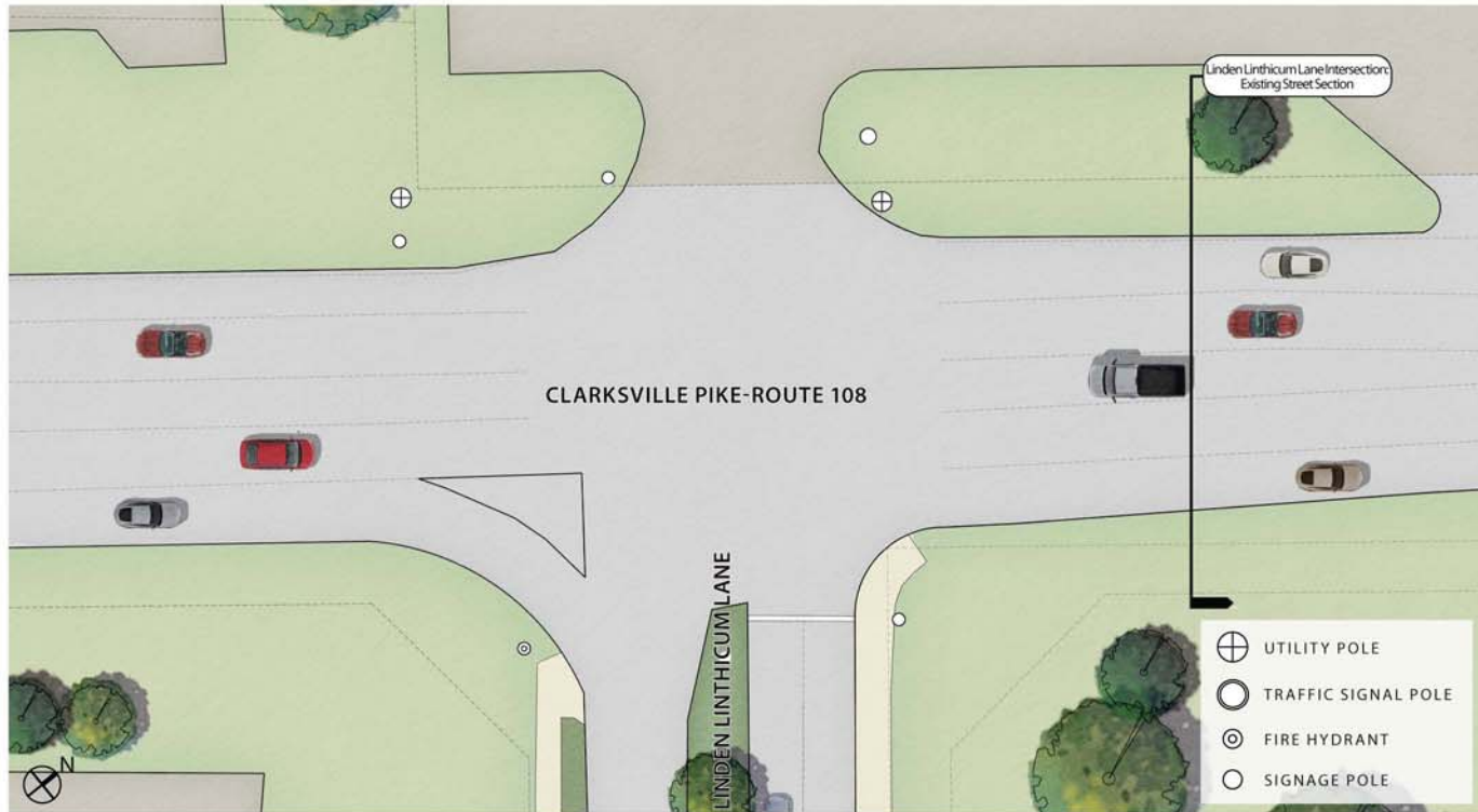
Existing Streetscape: The existing streetscape includes no sidewalks or crosswalks in this portion of Clarksville Pike. Landscaping is minimal.
