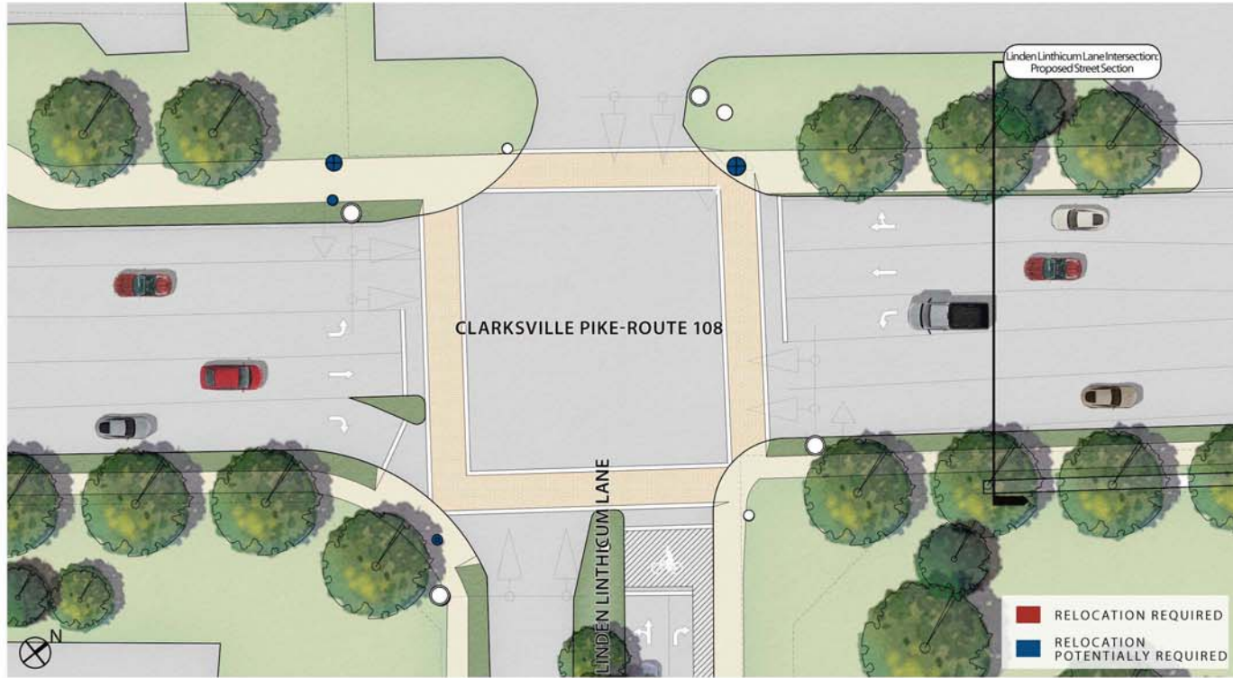
Proposed Streetscape: Streetscape improvements at Linden Linthicum Lane include crosswalks and ADA ramps, a continuous shared-use path along the western edge of Clarksville Pike, continuous sidewalks along the eastern edge and continuous planting strips and street trees on both sides. Bike accommodations along Linden Linthicum at the intersection of Clarksville Pike will be incorporated. Utility, signage, and traffic signal poles may need to be relocated.
