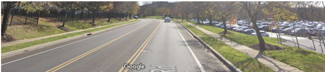
Striped median in southbound North Ridge Road. This area could be used to add a southbound lane, allowing the bus to stop in the far route southbound lane to provide more direct access to the Walmart entrance for pedestrians without blocking traffic.
