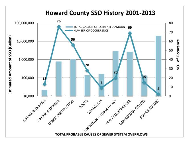
While taking the estimated overflow amount into consideration, power failure, storms, pipe and equipment failures rank the highest of the total SSO volume contribution. This observation has not changed from 2012.
