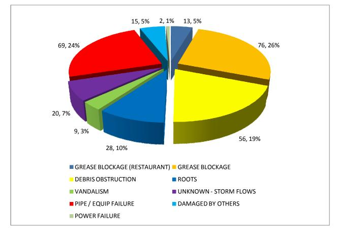
As is shown in the above chart, the top three (3) causes of overflows county-wise are: grease blockage (non FOG, 26%), pipe/equipment failure (24%), and debris obstruction (19%).
