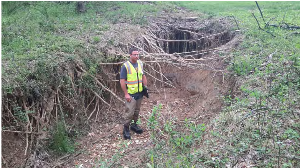
Facing upstream, a 7 ft. headcut moving from the stream to the pond.
