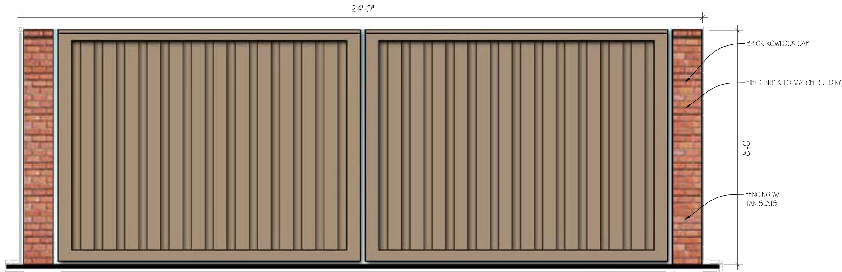
1 DUMPSTER ENCLOSURE REAR ELEVATION SCALE = 1/2" = 1'-0"
