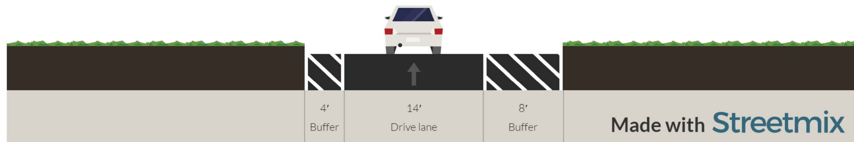
Existing Condition—Snowden River Parkway Ramp to Robert Fulton Drive (26' Existing Total Width)
