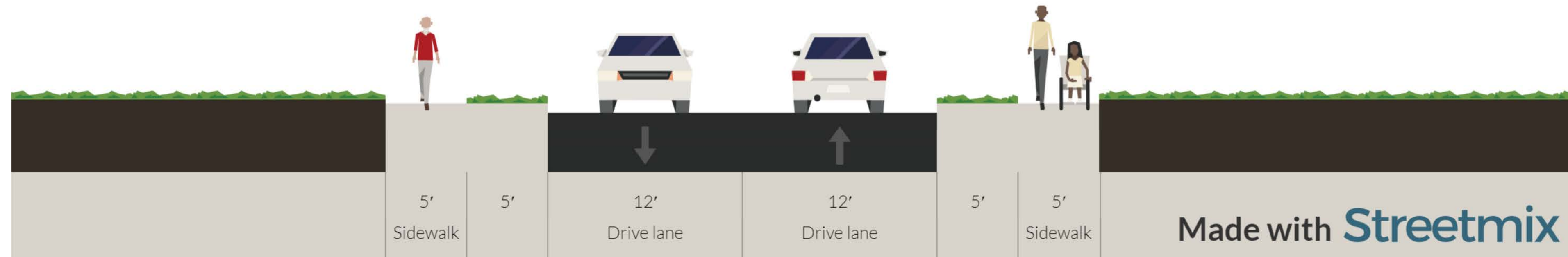
Existing Condition—Gracious End Court (44' Existing Total Width)
