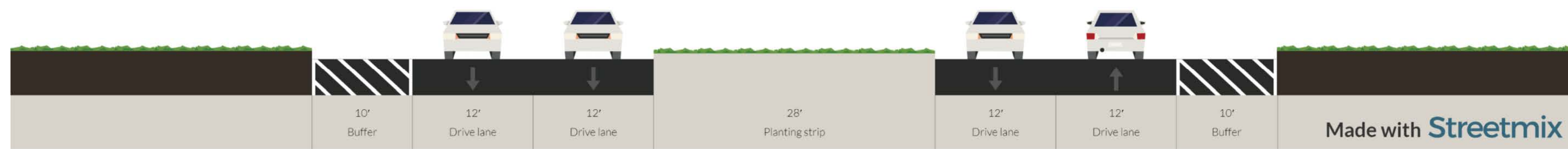
Existing Condition—Snowden River Parkway (96' Existing Total Width)
