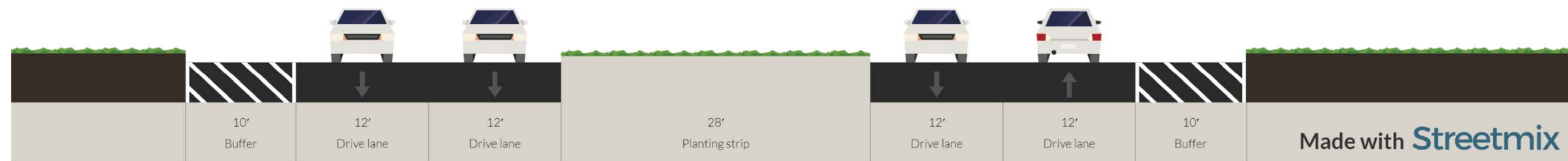
Existing Condition—Snowden River Parkway (96' Existing Total Width)
