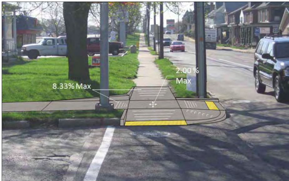
Re-configured curb ramp to provide two compliant ramps at the existing location.
