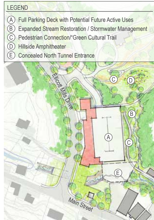
Figure 195: Lot F Full Parking Deck + Active Uses
